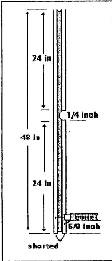
If you can do it cheap, I like it! This antenna is that and it works well, especially where space is limited.
